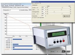
The AZ76 measures the temperatures of passing measuring objects with a pyrometer and determines their maximum temperature. These values are compared with a predetermined temperature range and supplies a corresponding control signal (via 4 switching outputs for the states overheated, too warm, good or too low) if temperatures are in accordance or deviation. Each measured value is stored in the device with evaluation result, date and time (max. 32000 records).
