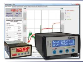
**Regulus** is a PID program controller (for panel-mounting or as a compact bench top model) optimized for use with pyrometers. Programming will be done via control software **SensorTools**, the program execution is performed completely self-sustaining by the Regulus.
