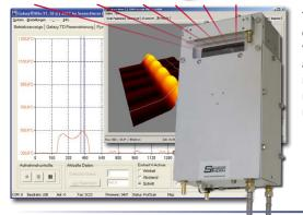
The line scanners **Galaxy SC11** and **SC12** steer the pyrometer's field of view continuously back and forth. They enable a linear line recording of measured values with recognition of critical temperature ranges. Scan angle and speed are adjustable.
