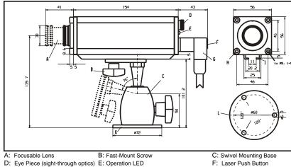
G: 12-pin Connector K: Swivel Base Mounting Flange
