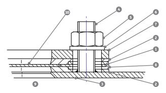
Installation with welded threaded bolts.
