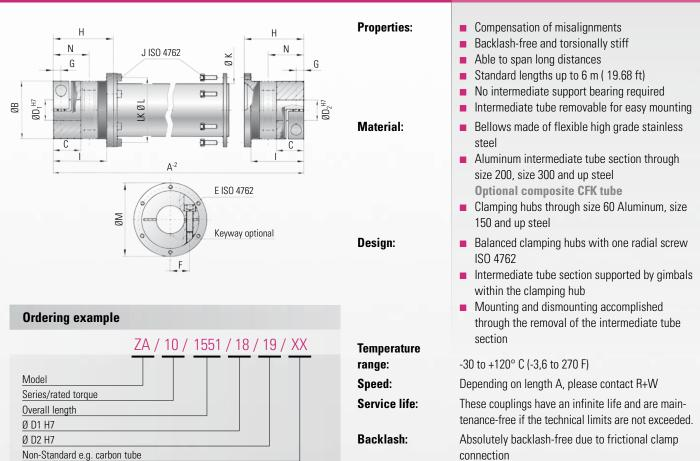
Shaft/hub connection 0.01 to 0.05 mm
