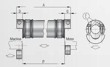
**Mounting:** Loosen Screw E and slide the metal bellows coupling segments onto each shaft end. Now insert the intermediate tube and assemble onto both metal bellows coupling segments using the assembly screws J. Tighten the assembly screws J to the correct torque indicated in the specification table. Center the entire line shaft coupling onto the shaft ends and tighten screw E by using a torque wrench to ensure the correct torque as indicated in the specification table.
